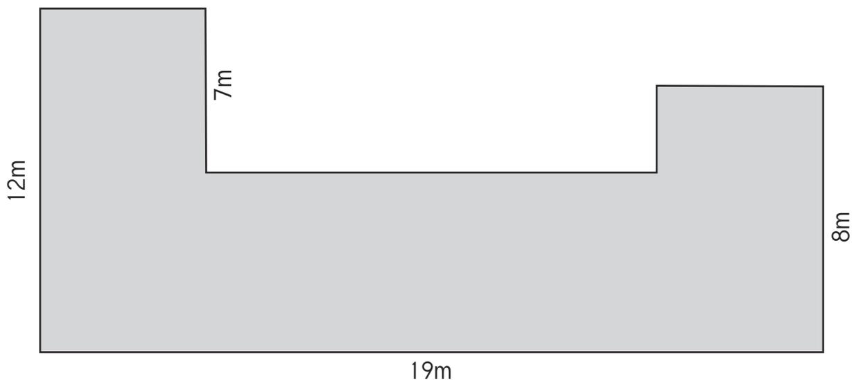
With this example the length of the 3 horizontal sides at the top will be 19m. There is one unknown vertical side. Because  $7\text{m} + 8\text{m}$  is 3m longer than the 12m on the left hand side, the unknown vertical side is 3m. These measurements can be used to calculate the whole perimeter as 68m.
